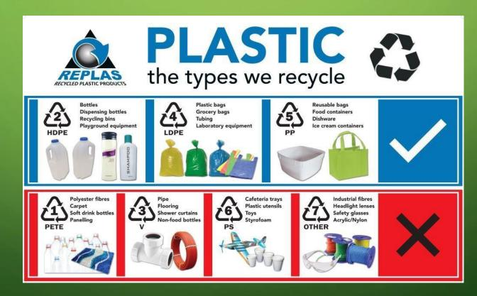
The main types of plastic include PET (polyethylene terephthalate), PE (polyethylene), PVC (polyvinyl chloride), PP (polypropylene), PS (polystyrene) and ABS (acrylonitrile butadiene styrene).
